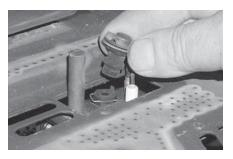
Unscrew the pilot orifice with the Allen key and replace with the LPG pilot orifice in the kit and replace pilot cap.
